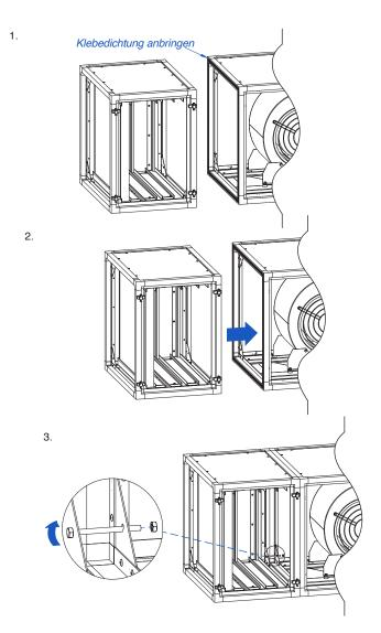
The screw connection system is already integrated in the Compakt fan type CLC, filter box type FB and activated carbon module type WAM series. **The W-Connect Kit must be used with the GBV and GBG airboxes.**
