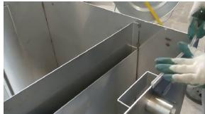
Put the lip seal on the edge all the way to the around and to the starting point
