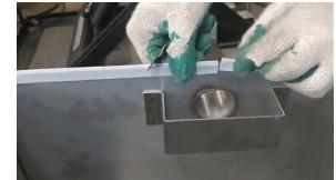
Remove excess silicone, put the cover back on firmly and close the quick-release fasteners
